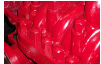
A 3x4-10 Series 380 OSMH pump in assembly
