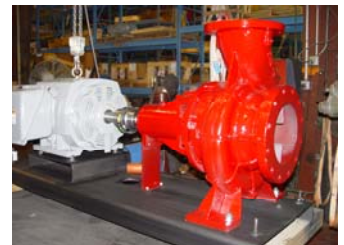
An 8x10-13 Series 300 REF pump in assembly
