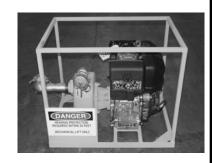
The heart of the system, the fluid end, is based off of the time tested NOVO 1.5" LSE process pump product line. This pump was originally designed to pump a wide variety of demanding process fluids. Due to these demanding applications, the casing, impeller and rear cover feature heavy wall construction extending the life of the parts. The rear cover is engineered to maximize seal life by self venting gases and ensuring a consistent and debris free stream of clean fluid for lubrication.
