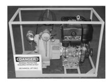
The heart of the system, the fluid end, is based off of the time tested NOVO 2" SPPAE process pump product line. This pump was originally designed to pump a wide variety of demanding process fluids. Due to these demanding applications, the casing, impeller and rear cover feature heavy wall construction extending the life of the parts. The rear cover is engineered to maximize seal life by self venting gases and ensuring a consistent and debris free stream of clean fluid for lubrication.
